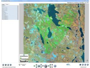
The area is between Sundsvall and Östersund. Both datasets were captured with 50 cm resolution. The area covered by GeoEye was 25\*25km. Leica ADS 80 covered a little larger area.
