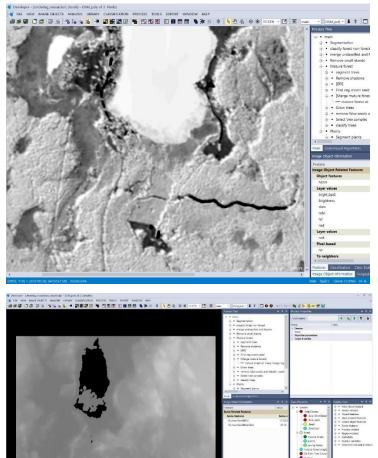
This terrain analysis shows different terrain formations. Dark lots are streams, ditches and recesses in the terrain. Elevations and dots become bright. Flat areas become neutral. Together with the presentation of deciduous trees, you can create maps showing moisture areas in the terrain.
